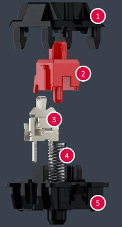
**1. Upper Housing** is a CAD high precision component made of plastic polymer ensuring precise movement of stem
